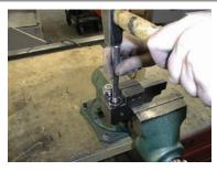
7. Install eccentrics to the cubes. Install components on both eccentrics in given order. Put bearings by means of the preparation on eccentrics.
