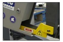
Install the yellow protective cover of the band. The arrow on the cover must match the direction of the arrow on the band. If it does not, you must turn the band
