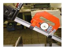
Stretch the saw band until it is stretched to the recommended value
