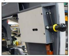
The saw band run is set with screw in the stretching cube on the saw frame. Optimal distance has been determined at **1 – 3 mm**.
