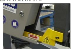
After the machine has been successfully connected, briefly switch on the machine and put the driving engine of the band in the running position. The direction must be in accordance with the arrow direction on the saw band cover. In case the direction of the saw band does not match, two phases at the terminal strip must be switched.
