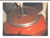
9. Put the wheel on the shaft and screw on the preparation to the wheel stretching to the hole in the shaft.
