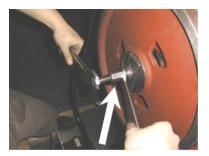
Screw on the preparation to the wheel stretching to the hole in the shaft. Pull on the wheel on the shaft.
