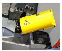
Never switch on the saw band drive if this cover is not mounted!
