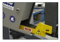
Never switch on the saw band drive if this cover is not mounted!
