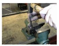
5. Remove eccentrics from bearings by means of the swager
