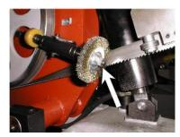
1. Release the nut of the brush, exchange old brush to new brush and screw on the nut of the brush.
