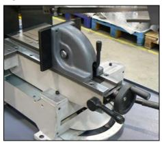
Release the clamping lever, shift the vice ca. 5 mm from the material and clamp the material to the vice by lever.
