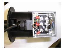
Remove the cover of the pump terminal switchboard. Disconnect 4 terminal connectors of the input cables. Cables are identified according to the red clamps..
