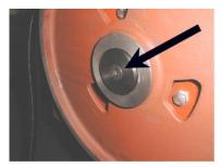
2. Screw off the screw and remove the washer.
