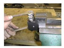
Tighten the guiding cube to the vice and dismantle both eccentrics with bearings following way.
