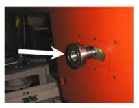
6. Install bearing on the shaft and move it to the retaining ring. Insert the distance ring on the shaft and move it to the bearing.
