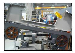
**The band saw is stated to the operation, when the covers is closed!** Limit switche on saw arm control if cowers are open or not.
