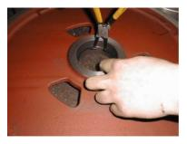
7. Insert the retaining ring to the hole in the wheel.
