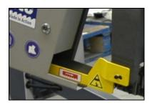
2. Dismantle yellow protective cover of the saw band. The cover is clamped with two screws.
